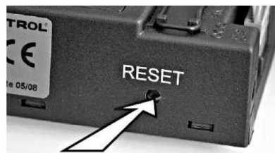
Fig. 10 - Receiver "RESET" button
